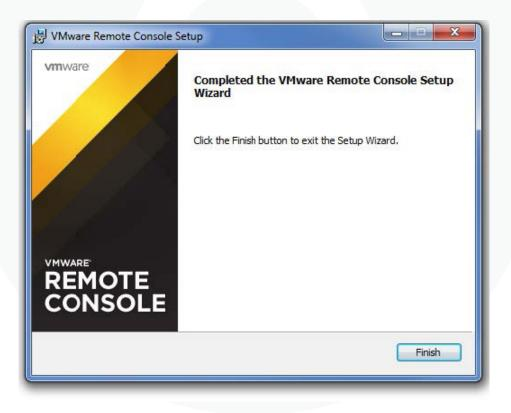
4. Press the Finish button. VMRC does not have a desktop icon, but you can check to make sure it installed correctly by opening your Control Panel and navigating to Programs and Features (Windows).
